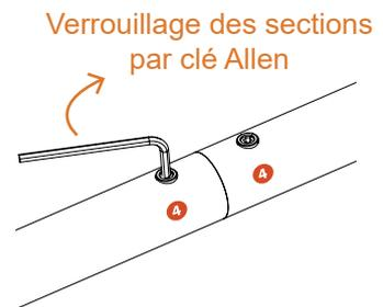
**ASSEMBLAGE DES SECTION DE LA STRUCTURE DE 30 MM**
